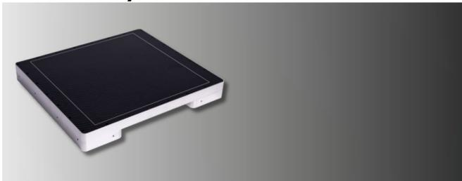
The 3131HS is a high speed dynamic X-ray detector designed for industrial applications, with a pixel pitch of 100  $\mu$ m and a choice of high-efficiency or high resolution Csl scintillator or Gadox. It is ideal for CBCT and AXI.
