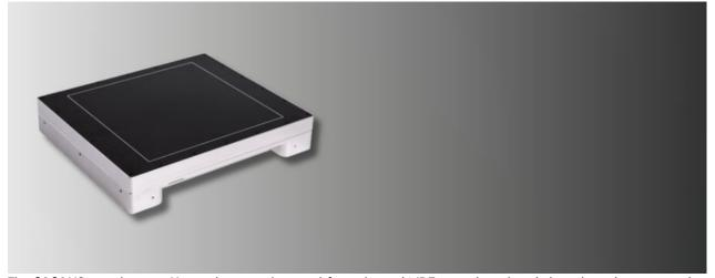
The 2121HS is a dynamic X-ray detector designed for industrial NDT, pre-clinical and clinical applications, with a pixel pitch of 100  $\mu$ m and a choice of high-efficiency Csl or Gadox scintillator. It is ideal for CBCT or fluoroscopy.
