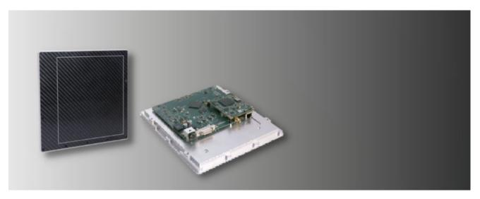
The 1615HS is a dynamic X-ray detector designed for dental, pre-clinical and clinical applications, with a pixel pitch of 100 µm and a choice of high-efficiency CsI or Gadox scintillator. It is ideal for CBCT or fluoroscopy.
