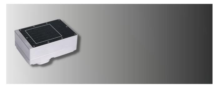
The 0606HR is a dynamic X-ray detector designed for industrial NDT, electronics inspection and pre-clinical applications, with a pixel pitch of 50  $\mu$ m and a choice of high-resolution Csl or Gadox scintillator. It is ideal for CBCT and real-time inspection.
